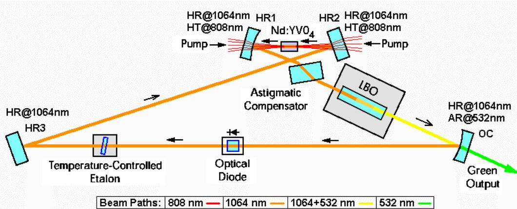
Ring Cavity Resonator of Coherent, Inc. Verdi Green DPSS Laser
