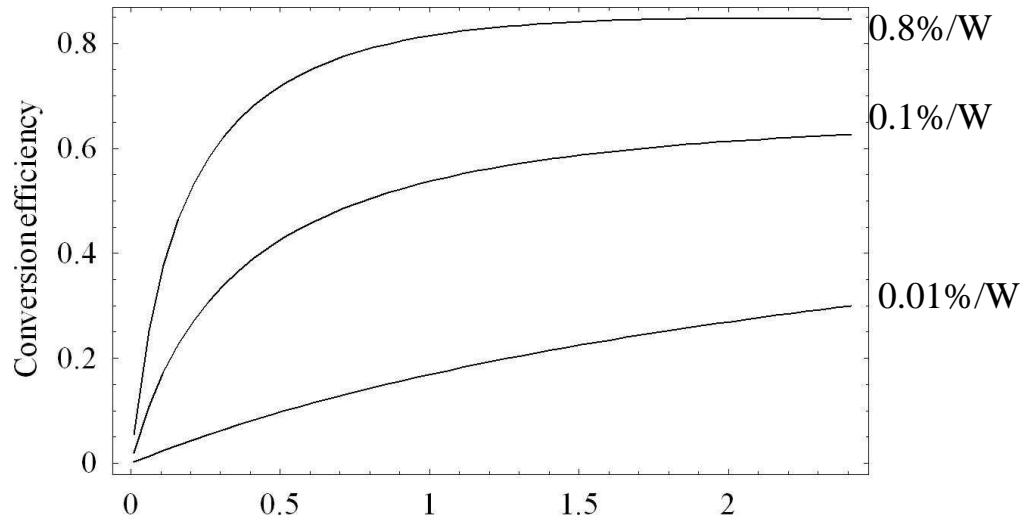
Efficiency vs. losses in the cavity.
