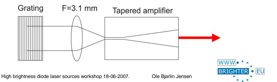
DTU The tapered laser - results
