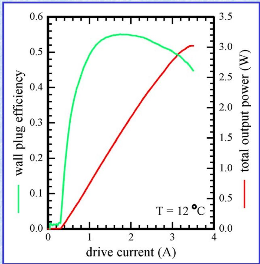
wall-plug efficiency up to 55 % at 1.5 W
