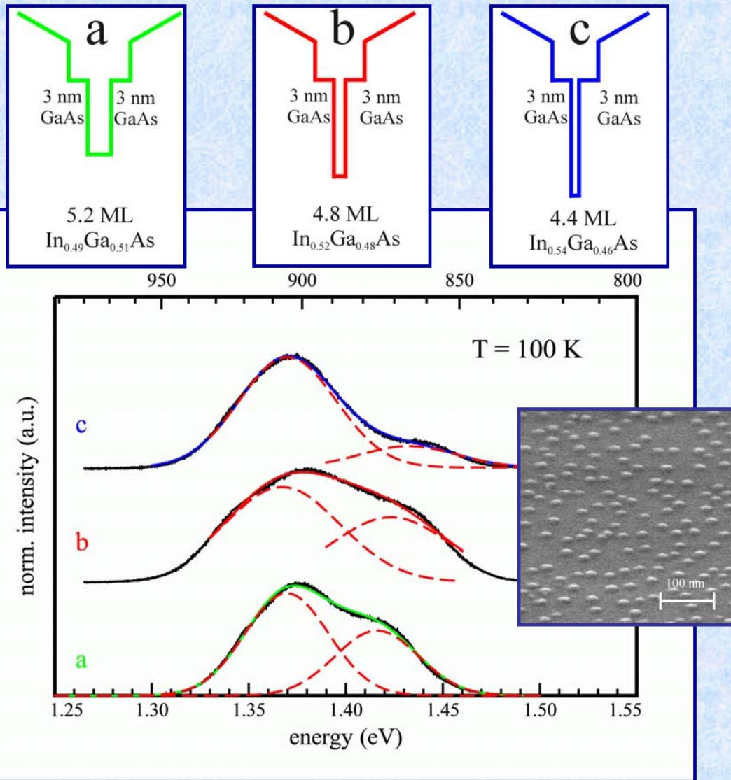
**Photoluminescence measurement of different QD samples at high excitation powers:**
