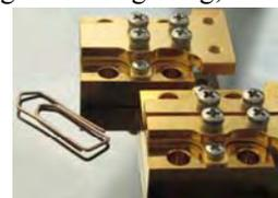
*Above: Photograph of a mounted dual contact DBR tapered laser.*
