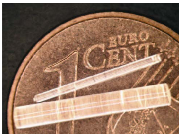
Figure 1: Plane aspheric fast axis collimators with different focal length
