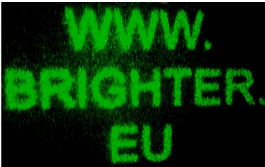
Fig. 2 Replay of hologram in holographic projector using green laser from ILT
