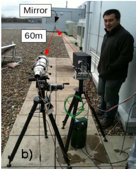
Free space transmitter and receiver carrying out outside FSO link test on roof of CAPE building Received 1.25Gb/s eye diagram after 60m link
