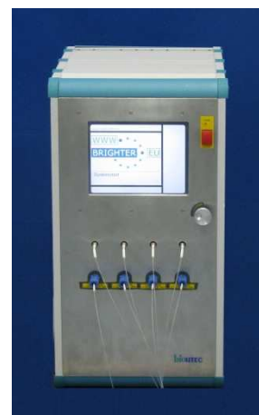
Figure 1: The photo shows the iPDT system. It has 4 laser ports in the lower row of SMA connectors and 4 detection ports (upper row of SMA connectors).
