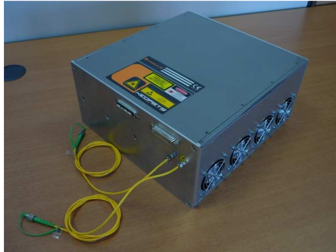
Kéopsys Cladding Pumped EDFA prototype
