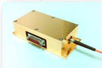
200 \mu\text{m} fiber coupled Module (IDs 4.3.3,4.3.5,4.3.6)
